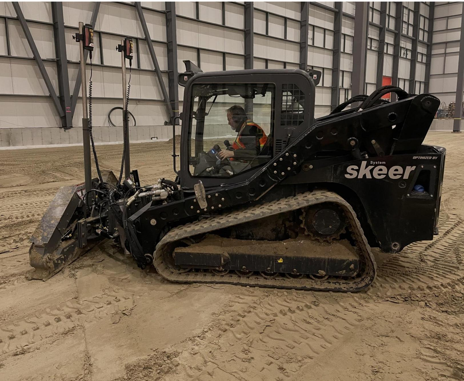
The Leica iCON grade iGD2 solution provides automatic control of both slope and elevation. Laser receivers are mounted on the dozer and used together with a rotating laser. A single laser indicates height. Adding an extra mast and laser sensor allows you to work independently of the slope direction.
