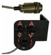
EG Series Remote Toggle Switch Assy: You can switch your EG2 from auto to manual mode, or raise and lower the valves right from the lever in your cab. The switch on the bottom toggles the EG Series between Automatic and Manual mode, and the switch on the top raises and lowers the valves. The switch assembly attaches to any lever using the universal U-bolt assembly.
